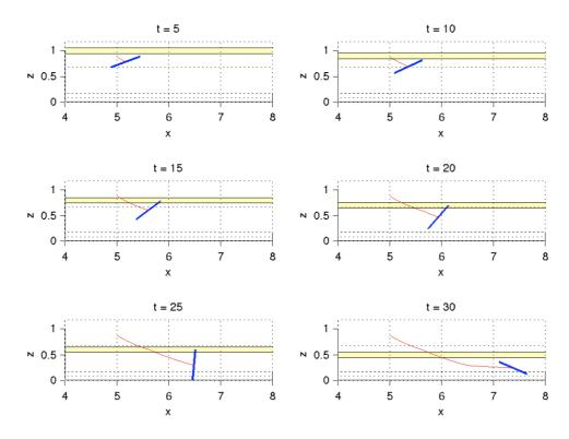
**Figure 2:** Evolution of the position and orientation of a short fibre immersed in a squeeze flow and interacting with the upper gap wall.
